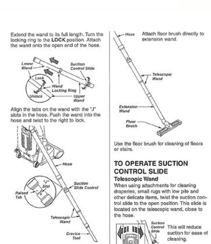
attachments, add the crevice tool to the end of the wand by inserting and twisting slightly. The combination brush can be attached directly to the wand.
